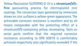
good corrosion behaviour and good thermal stability. It's characterized by a wide field of operation
